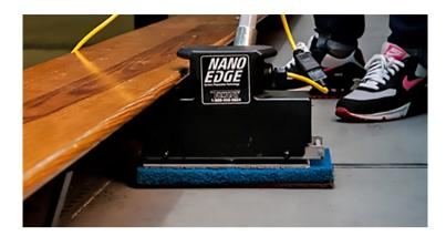
Its compact sizes enables it to clean better in areas where bigger scrubbing machines can't reach. And it's powerful too, scrubbing at 4100 RPM, removing dirt quickly and with ease. It's also perfect for scrubbing staircases.
